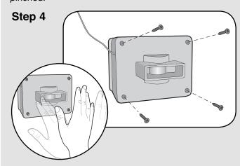
Test PIR Motion Sensor by waving hand in front of sensor. Test light should flash. Secure cover with the smallest screws.
